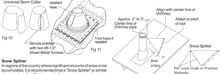
device be installed. This is especially important on metal or steep sloped roofs. A Snow Splitter helps protect the chimney and the roof flashing from damages caused by sliding snow or ice by diverting it around the roof flashing and the chimney.
